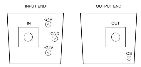
The input and output SMA connectors are located on opposite ends of the module, as shown above.
